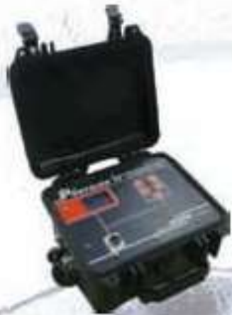
Ultrasonic Flow meter for water and sewage (EESIFLO capable of measuring flow in pipes up to DN 2500 mm) – EESIFLO make
